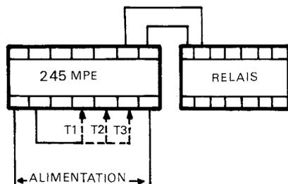
*When AC or DC is supplied to the module, the relay (or any load) switches on after the preset delay.*
