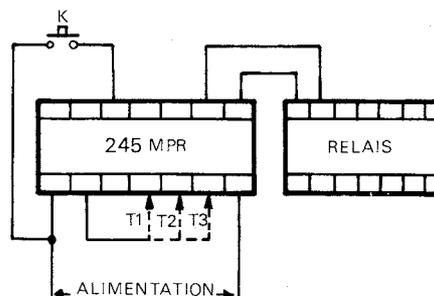
*The module must be AC or DC constantly supplied. When closing outer control K, relay contacts close. When opening K relay contacts open after the preset delay.*
